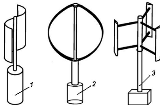
Fig. 1. Types of vertical axial wind turbines:
