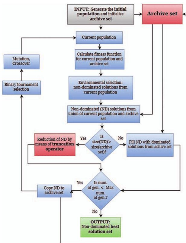
Fig. 3. Block scheme of SPEA2 algorithm
